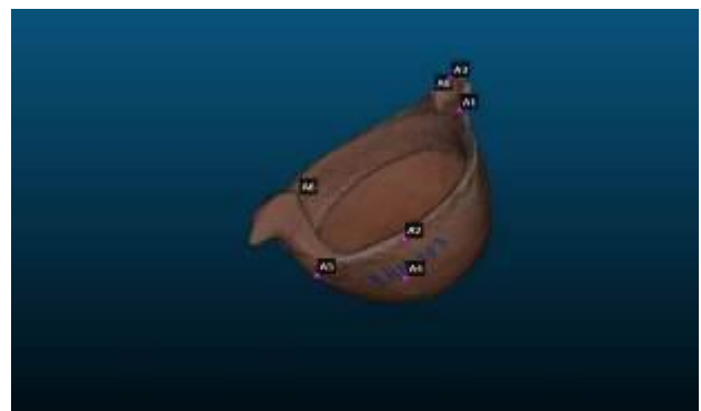
Figure 8: Point selection for the alignment of the compared meshes
