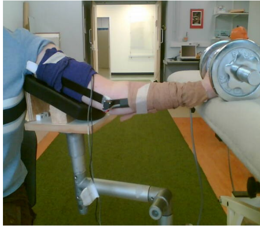
Figure 4.1. A eccentric-concentric contraction test. An electronic goniometry was attached at the fulcrum to measure elbow joint position. A bandage was used to ensure consistent pressure of the contact sensor.
