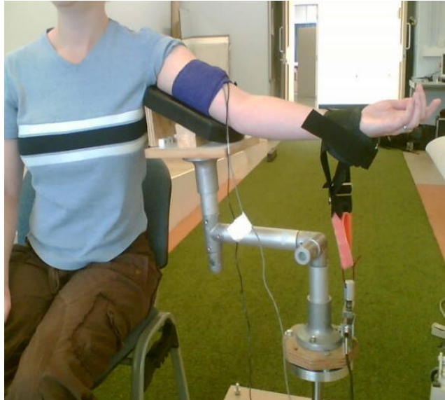
Figure 3.1. Isometric MVC test setup. Electromyographic (EMG) and mechanomyographic (MMG) sensor were placed in the middle line of biceps brachii. A bandage was used to ensure constant pressure of the sensors over the muscle.
