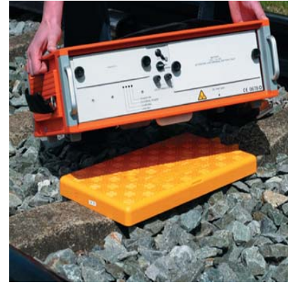
Figure 2.8.: Programming for a Eurobalise (Siemens AG, 2008a)
