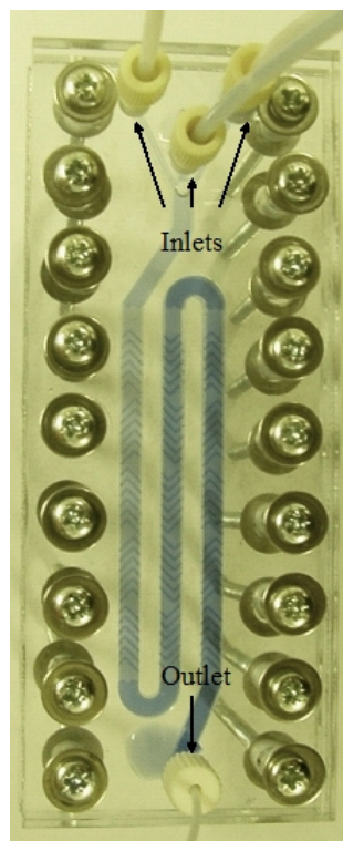
(c) Picture of the acrylic chip employing a layered herringbone channel. The chip is 60x150mm.
