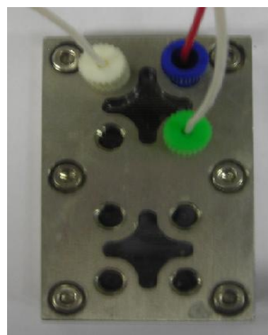
(b) 100x300 \mu\text{m} (width x depth) silicon/glass mixer channel with stainless steel holder
