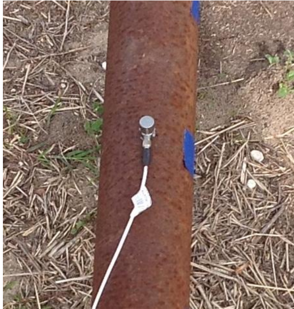
Figure 4.4: Accelerometer r-configuration measurements
