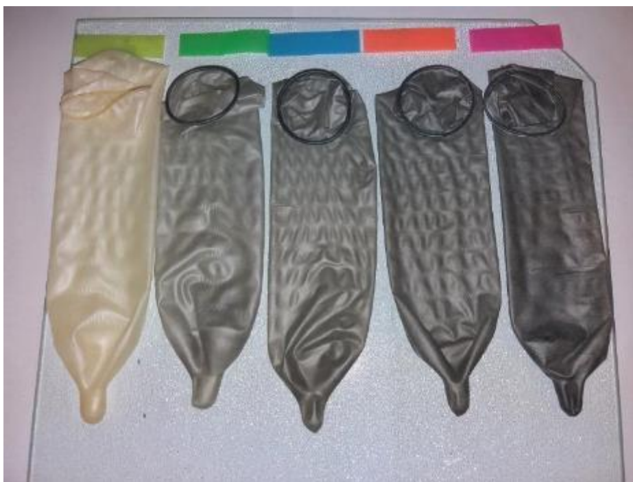
Figure 3.1.1.4: Samples of MLC produced using the different latex blends. From left to right; PvNRL, Pv-NB/1, Pv-NB/2, Pv-NB/3 and Pv-NB/4.
