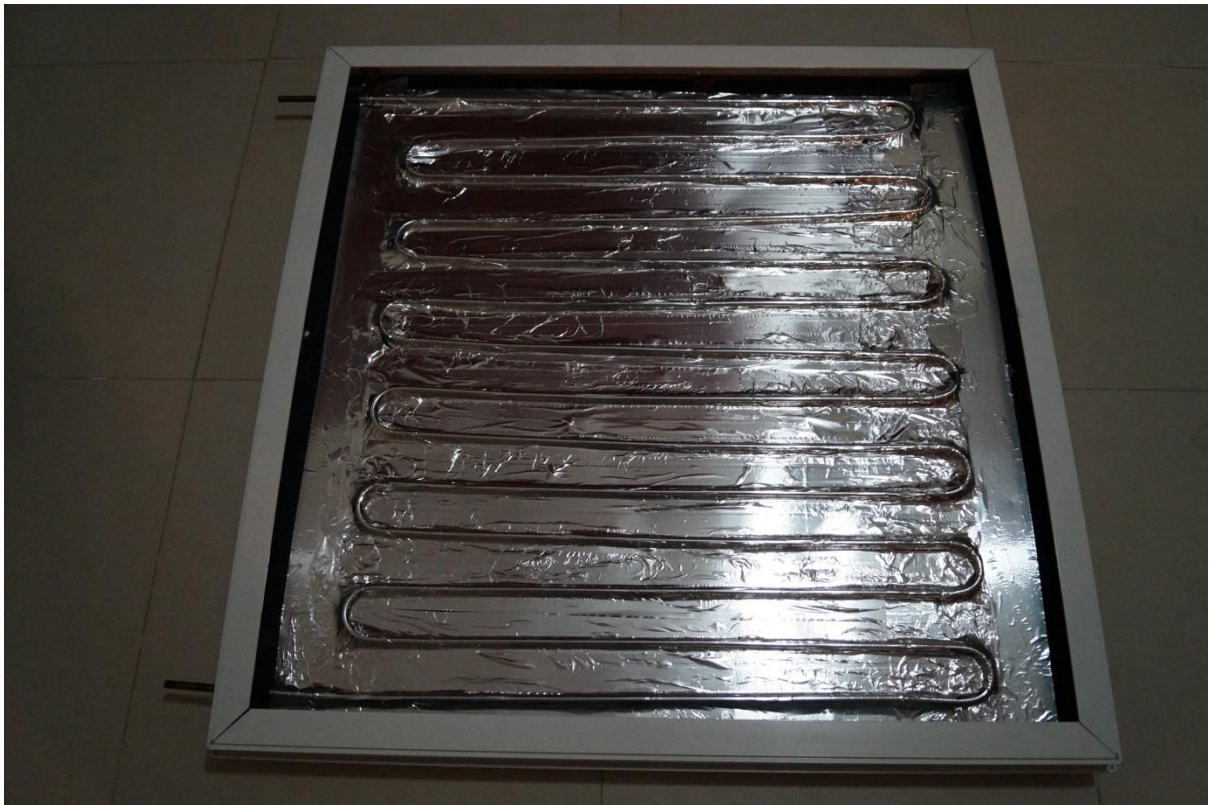
Photo 4.4 Edge Insulation Completed
