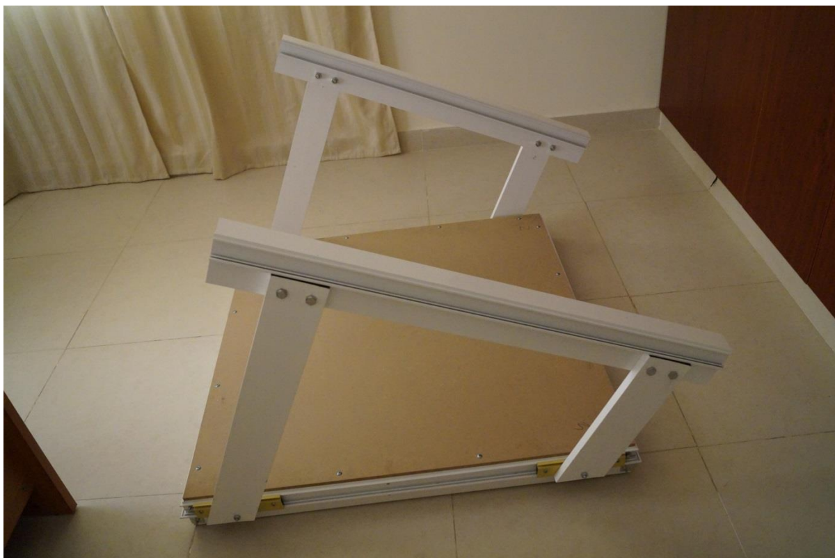
Photo 4.6 Underside Completed with Skids
