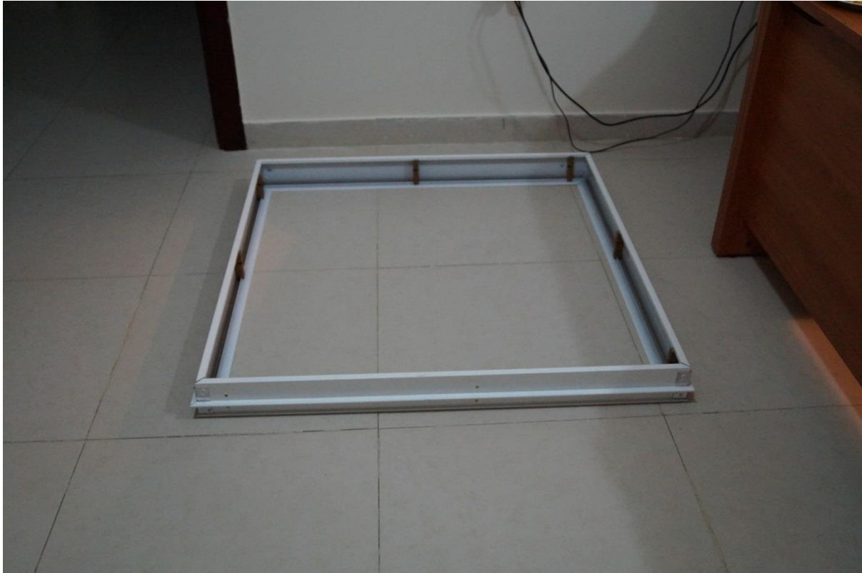
Photo 4.2 Wooden Cleats for Collector Frame Attachment
