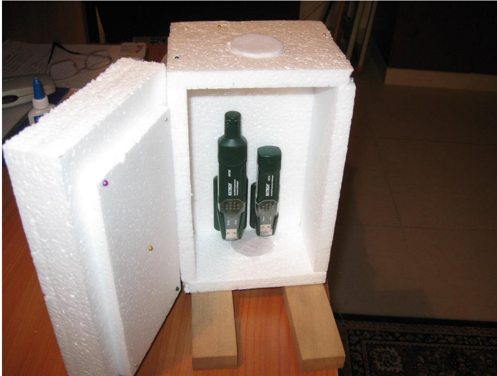
Figure 8.1: Meteorological Instrument Cabinet
