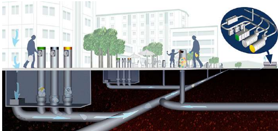
Figure 41 – ENVAC Self-Emptying Litterbins, (source: envacgroup.com, 2016)
