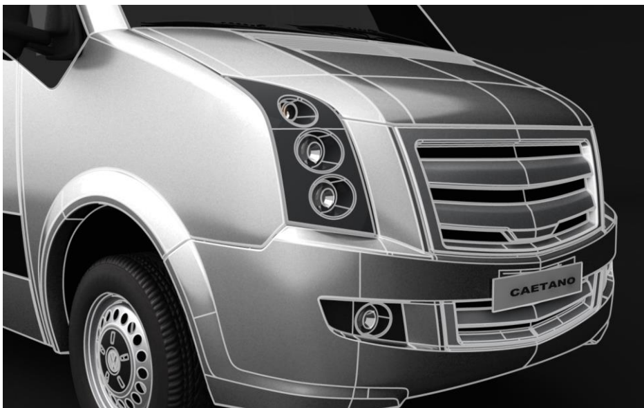
Figure 69 : 3D CAD surface model of a bus (source: Almadesign archive, 2010)
