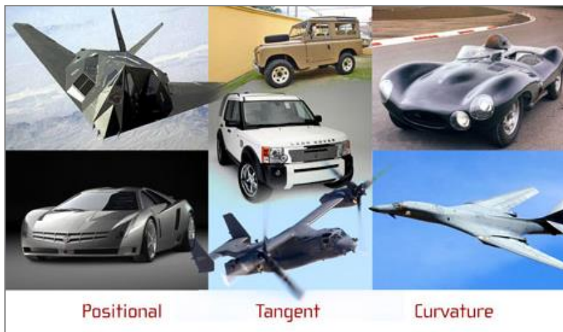
Figure 72 : Quality of surface transition in Transportation Design (source: Gray Holland, 2009) http://www.core77.com/posts/12752/a-periodic-table-of-form-the-secret-language-of-surface-and-meaning-in-product-design-by-gray-holland-12752 (Accessed: Jan.2016)
