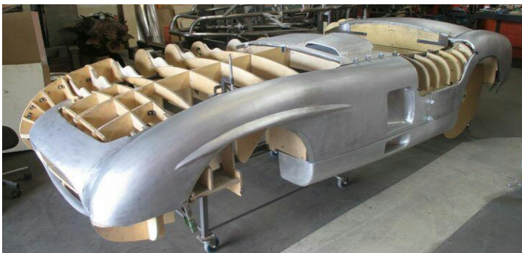
Figure 75 : Wood buck used to hammer steel and build the bodywork
