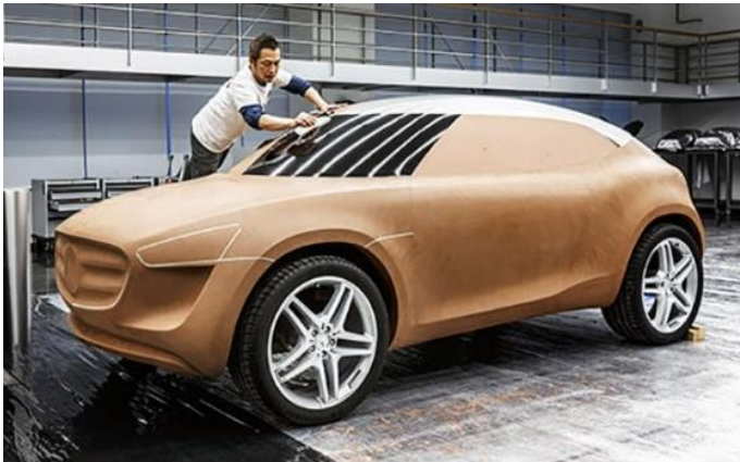
Figure 74 : Surface continuity and reflections - Mercedes Vision G-Code Concept
