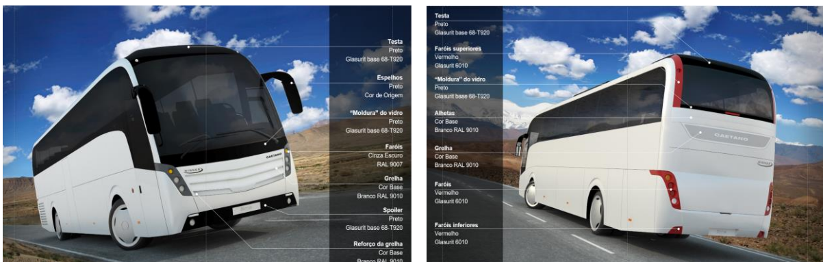
Figure 160 : Case Study #1: CMF details for production (source: Almadesign archive, 2012)
