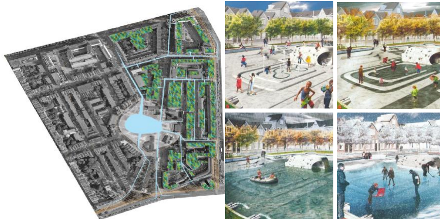
Figure 3 – Concept of Water Plaza in challenging flooding scenarios. Source: (Boer, Jorritsma and Peijpe, 2010)
