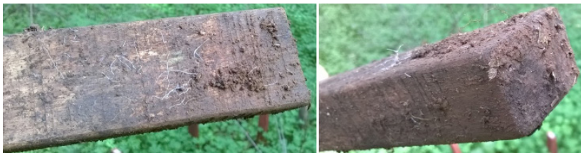
Figure 3. E. botryoides wood: images of the samples after ground contact.
