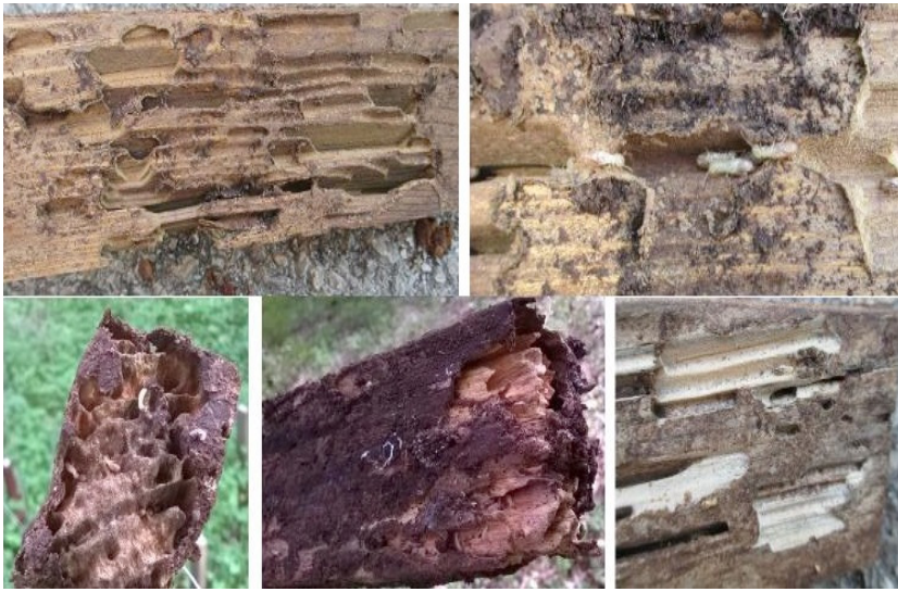
Figure 2. E. globulus wood: images of the samples after ground contact.
