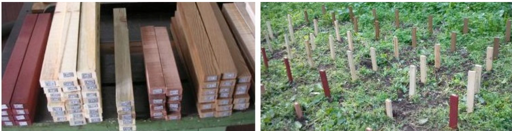
Figure 1. Field test for wood durability: preparation of the samples (left); samples placed in the ground according to EN 252:1989/AC1:1989 specifications.
