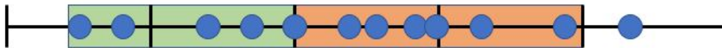
Figure 2.2: Example of a window pair for n_u = 5 and t_r = 60 minutes. Each vertical tick represents half an hour and each circle a node. u (green) begins at the first node and continues to include up to the fifth. r (orange) begins immediately after the fifth node and continues for one hour and in this case contains the next six nodes.
