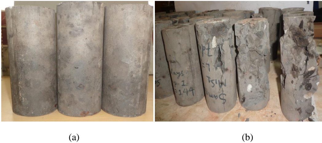
Figure 5.21: Cylindrical specimen samples (a) before the test and (b) after the test.
