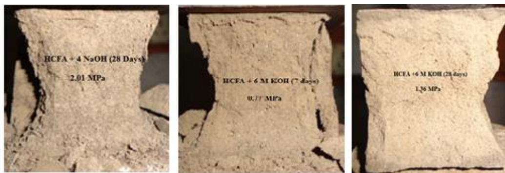
Figure 7.30: Failure pattern of alkali activated Paradeep fly ash.
