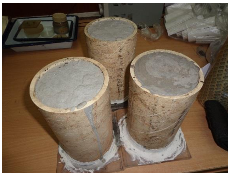
Figure 5.23: Settlement test set up for CLSM samples.
