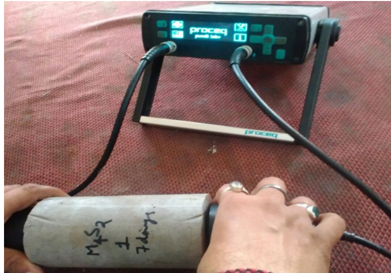
Figure 5.14: Ultrasonic pulse velocity measurement of CLSM sample.
