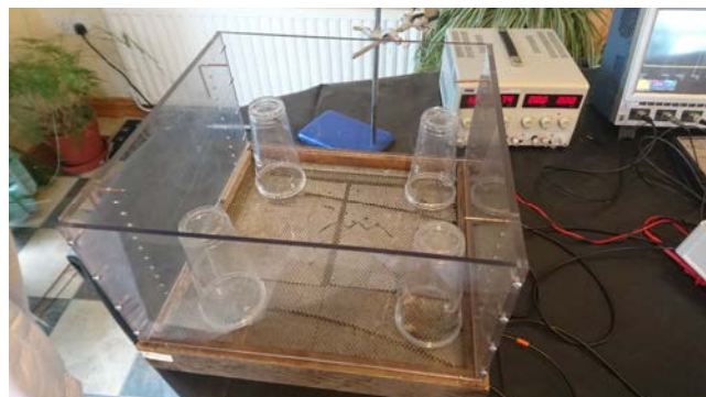
Fig. 3 Enclosures used for observation of bee behaviour during ultrasonic exposure.
