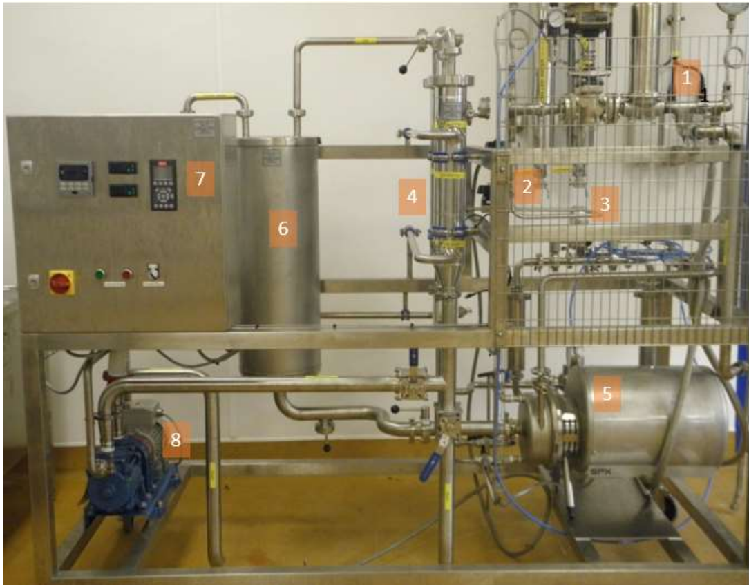
Fig. 5.1. SSIH process line where the main components of the line are shown; (1) steam supply and culinary steam filter, (2) SSIH injector, (3) holding tube, (4) flash vessel and condenser, (5) product return pump, (6) CIP tank, (7) control panel, and (8) vacuum pump.
