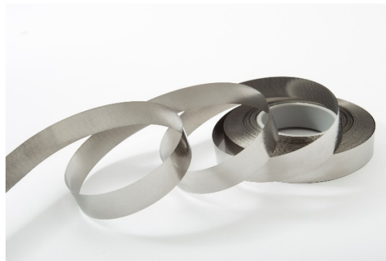
Fig. 6. Ribbon of amorphous soft magnetic alloy. Thin (5 to 50 \mu\text{m} ) ribbons of amorphous alloys are produced by planar flow casting.
