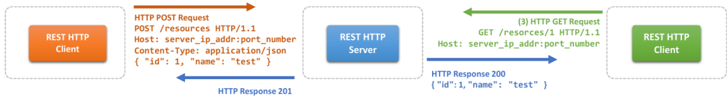
Fig. 4. REST HTTP interaction model
