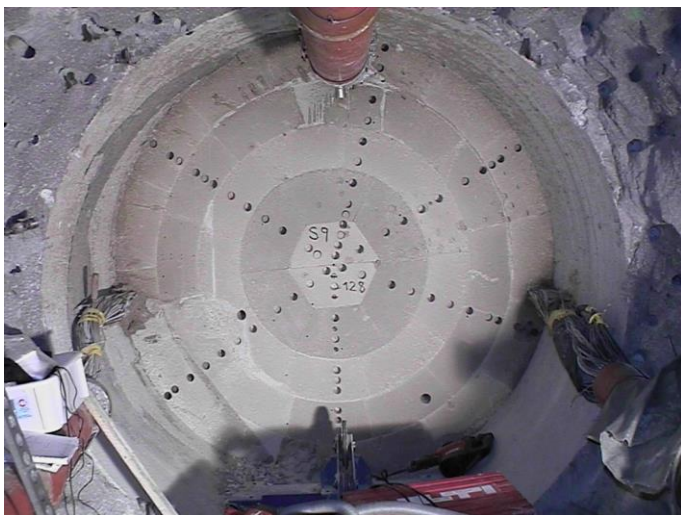
Figure 4. State of the barrier in the first dismantling. The location of the samples extracted from this section can be noted.
