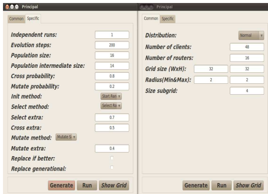
Fig. 5 GUI tool for WMN-GA system.
