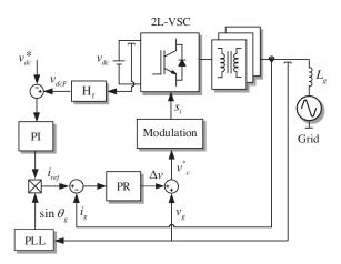
Fig. 5: Single-phase voltage oriented control scheme
