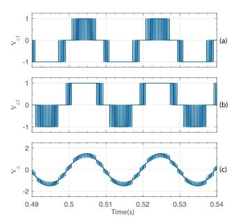
Fig. 6: Voltage waveforms. (a) Converter voltage  $v_{c1}$ , (b) Converter voltage  $v_{c2}$ , (c) Output voltage  $v_c$
