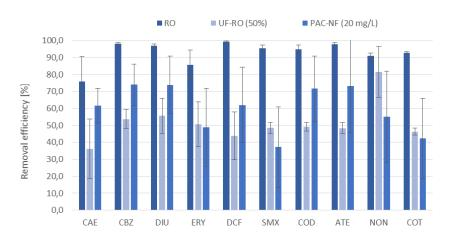
Figure 1 Comparison of OMP removal efficiencies between PAC-NF system and conventional advanced water reclamation systems RO & UF-RO(50%)
