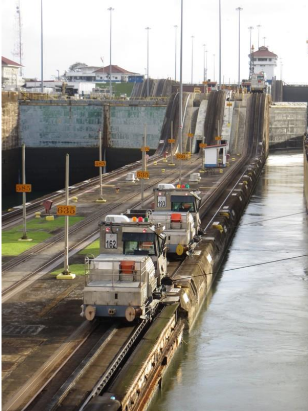
Fig. 1: Entry into the Gatún locks of the Panama Canal; vessel lead by mulis. (Foto: H. Auel)
