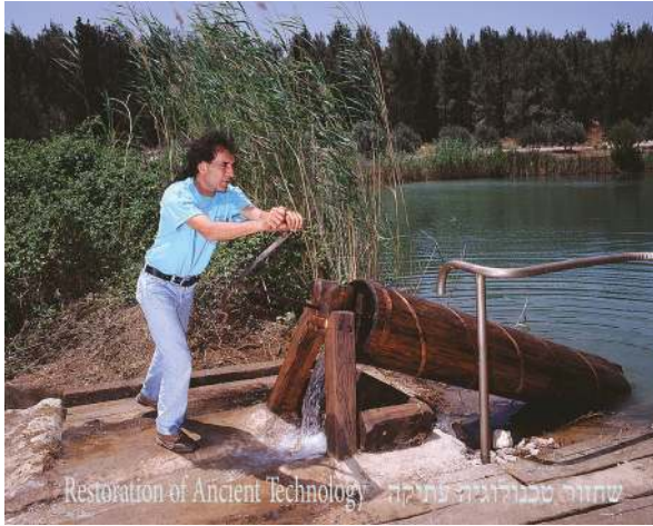
Fig. 1 A reconstructed Archimedean screw in Israel. This low-lift device has the advantage of draining quite a reasonable amount of water by a simple manual system. In antiquity, the device was turned with the feet. Photograph and reconstruction work, Yeshu Dray.
