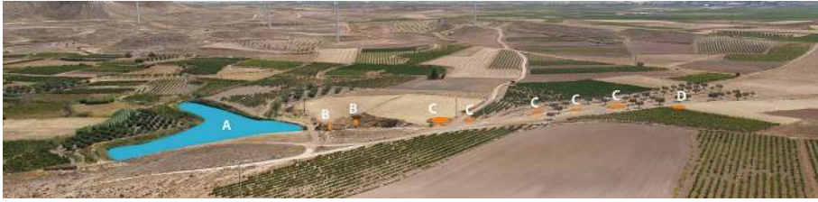
Fig. 11 The qanat at Bureta, Zaragoza, includes: (A) a pond, (B) outlets for the adit and qanat , (C) shafts, plus (D) the mother well.
