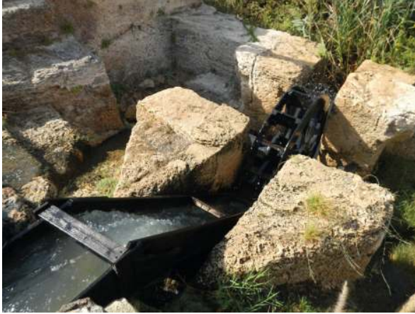
Fig. 9 Undershot wheel installation of a reconstructed Byzantine water mill at the river Nahal Tananim. This structure is a good example of ancient water-mills that still function.
