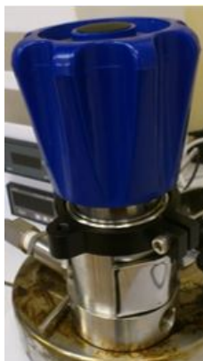
Figure 4.5: Pressure control valve.
