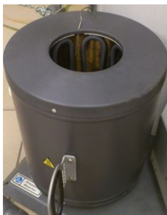
Figure 4.9: Oven for reactor temperature control.
