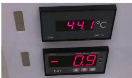
Figure 4.6: Digital screens giving the values of temperature ( ^{\circ}\text{C} ) and pressure (bar).
