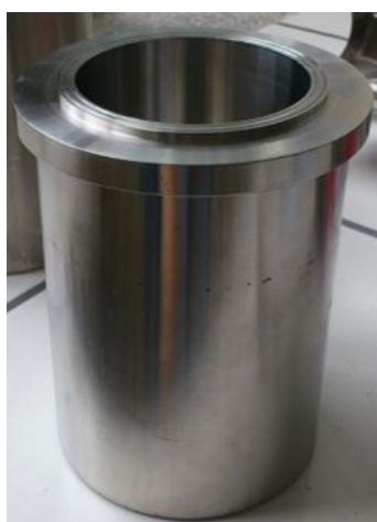
Figure 4.8: Type of reactor used in static extraction.
