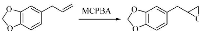
Figure 3.6: Epoxidation of safrole using MCPBA has an oxidizing agent.
