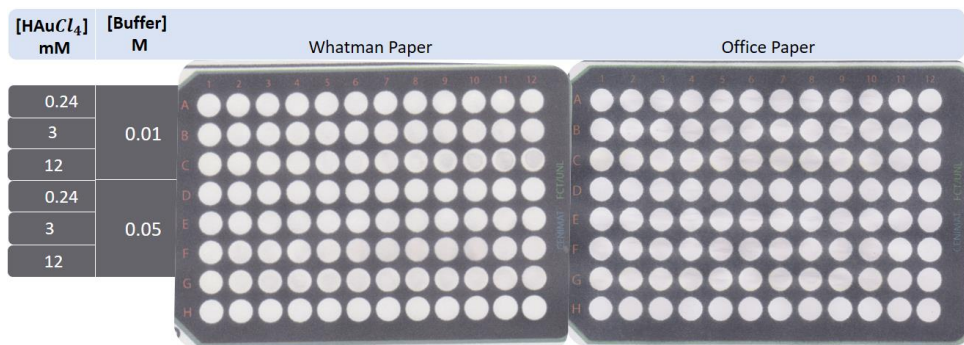
Figure 3.8- Synthesis of AuNPs on paper by reduction with TC, performed on a 96-well microplate on Whatman and Office papers.
