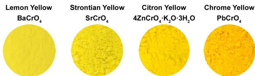
Figure 3.18. The final colour of Lemon Yellow ( \text{BaCrO}_4 ), Strontian Yellow ( \text{SrCrO}_4 ), Citron Yellow ( 4\text{ZnCrO}_4 \cdot \text{K}_2\text{O} \cdot 3\text{H}_2\text{O} ), and pure chrome yellow ( \text{PbCrO}_4 ) manufactured following W&N 19 th century recipes.
