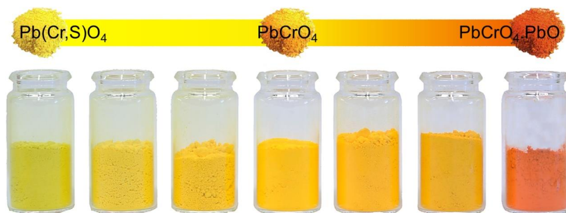
Figure 3.5. The final colour is modulated by pH during manufacture. On the left: the lemony mixed crystals of lead chromate and lead sulfate that precipitate at low pH; centre: the yellow pure lead chromate monoclinic phase ( \text{PbCrO}_4 ) at neutral pH; on the right: an orange/red basic lead chromate ( \text{Pb}_2\text{CrO}_5 ) formed in basic media.
