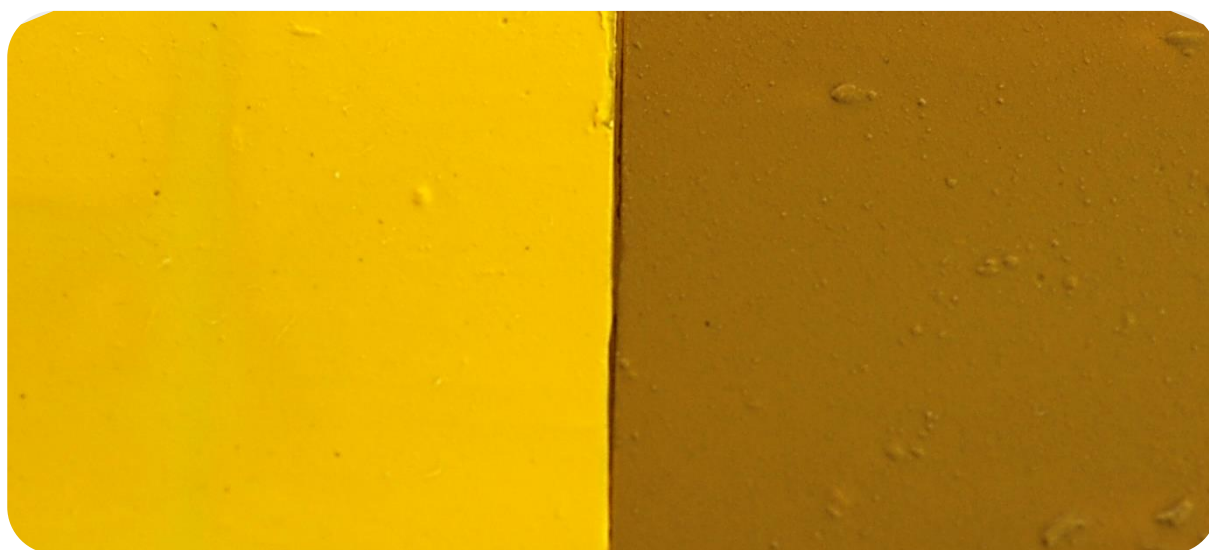
Image of a chrome yellow paint before and after Xenon irradiation @ DCR FCT NOVA
