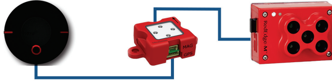
Figure 4.8: Micasense integration between Rededge-M, GPS module and DLS sensor.
