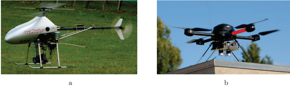
Figure 2.6: (a) Helicopter based Mini-UAV by weControl (Zurich), from [10]. (b) Quadcopter micro-UAV 'microdrones md4-200', from [10].
