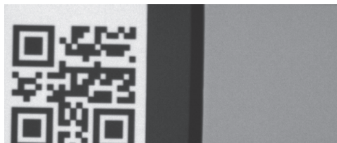
Figure 5.2: Calibration's panel base image with the QRcode and radiance square to use on automatic detection procedures.
