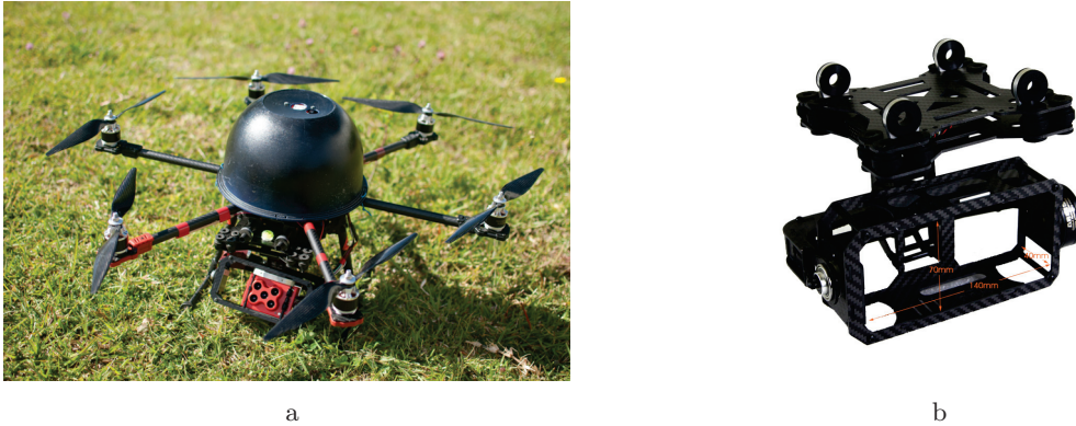
Figure 4.9: UAV infrastructure: (a) Model infrastructure of the Micasense camera integration with the UAV. (b) ARRIS ZHAOYUN pro 3-Axis Brushless Gimbal 32bit Version.
