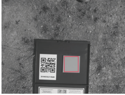
Figure 4.11: Calibration panel captured by the RedEdge-M NIR sensor in use.
