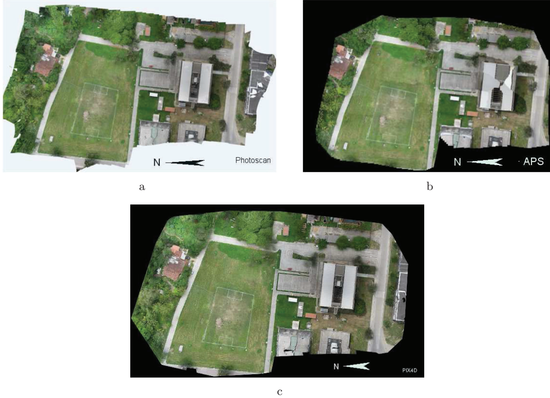
Figure 2.10: Software orthomosaicking results by: (a) Photoscan, (b) APS and (c) Pix4Dmapper. Illustrations from [24].
