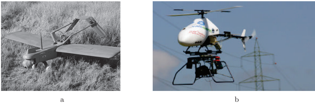
Figure 2.5: (a) Fixed-wing aircraft (BAT 3 UAS), from [8]. (b) Remotely Controlled Helicopters (RC-Helicopter) by Helicam and weControl, Switzerland, from [9].
