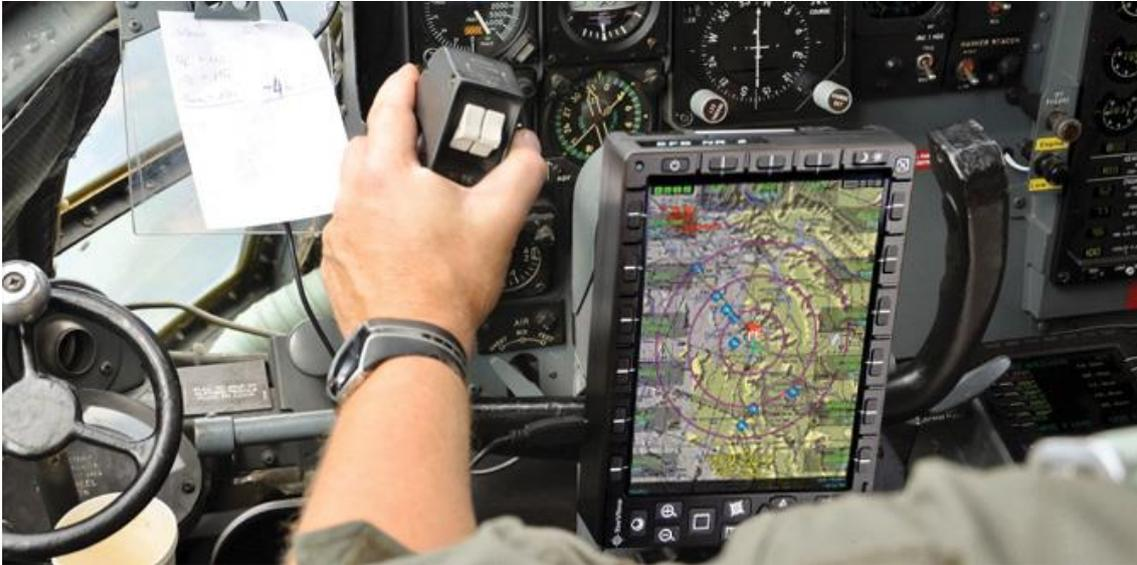
Figura 77 – Eletronic Flight Bag
