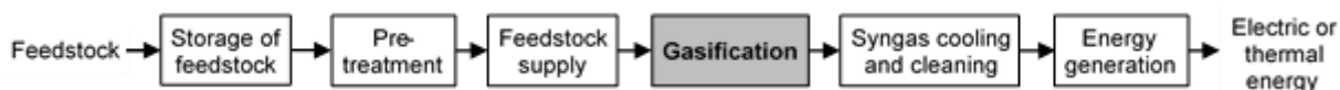
Figure 1. Main stages of a gasification plant (adapted from European Commission, n.d., p. 12).
