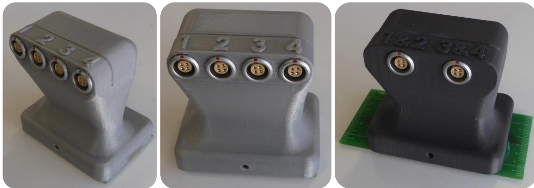
Figure 5.30 – PCB probes assembled in the 3D printed chassis.
