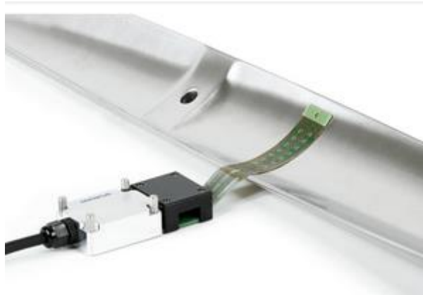
Figure 2.10 – Flexible eddy current array probe [133].
