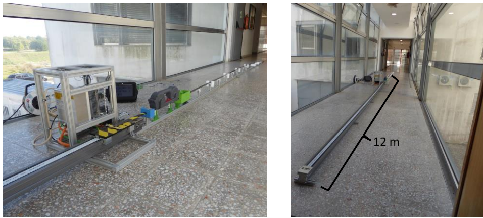
Figure 5.17 – Set up for the high-speed inspection with the linear guide and the CFRP guiding structure.
