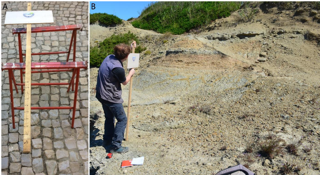
Figure 22: Jacob's bar (A) and its use in the field (B).
