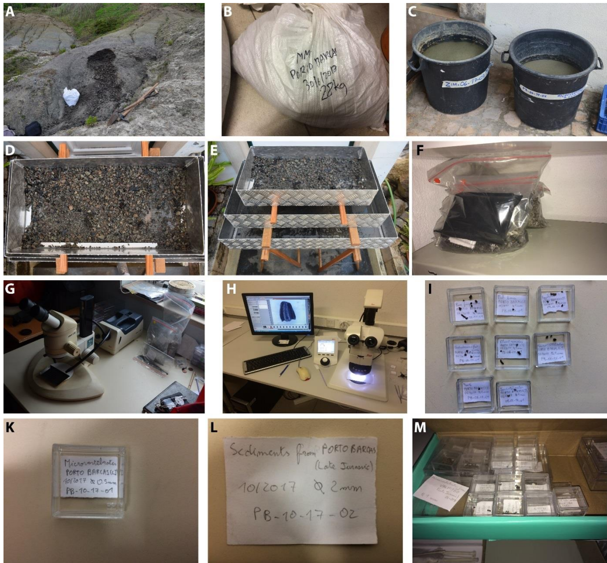
Figure 21: The different setups for preparation of the sediments. A , collecting in the field (Porto Barcas locality, 14/06/2018); B , bulk sample collected; C , bulk samples soaking in hydrogen peroxide; D and E , sieve table with 2mm, 1mm and 0.5mm meshes; F , plastic bags used to store sediments once they have been screen washed; G and H , binocular lenses in the Museu da Lourinhã ( G ) and FCT facilities equipped with a camera ( H ); I , sample boxes used for organizing specimens according to their locality, their description and their taxonomic identification; K and L , labels used to identify specimen boxes ( K ) and sediments screen washed ( L ); M , boxes used for the storage and the transport of the specimens.
