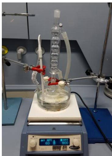
Figure 5: Amino-functionalized silica nanoparticles synthesis setup.
