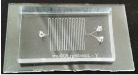
Figure 12 Complete droplet generator, Y-Junction in this case. An individual photo of all droplet generator chips can be found in Appendix D.
