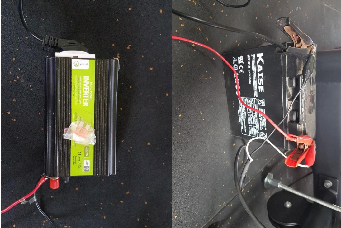
Figure 4.6 - Inverter (left) and battery (right) used in the preliminary tests of the motion harvesting system
