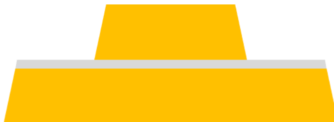
Figure 4.1 - Schematic cross-section of the final structure. A thin layer (3 nm) of \text{Al}_2\text{O}_3 (in grey) sandwiched by a big (120 nm diameter) bottom Au disk and a small (55 nm diameter) Au small disk, both having a 20 nm height (both in orange).
