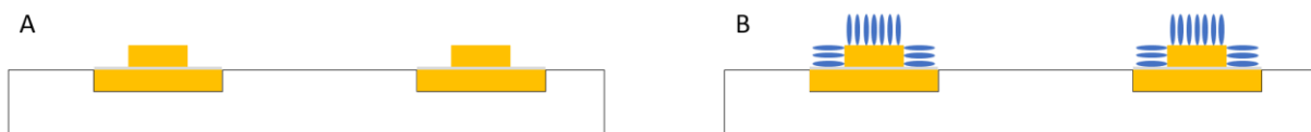
Figure 1.1 – A) Cross section of the ideal structures to be developed. B) Cross section of the structures with proteins (in blue) to be detected bound only to the upper disk.
