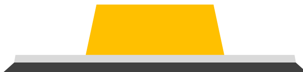
Figure 4.5 - Schematic of the small disk fabrication. The materials used are the same except the bottom disk, which is 3.9 nm high SiO 2 (depicted in black) instead of Au.
