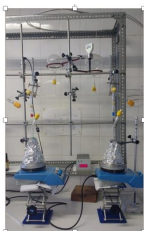
Figure 15. Assembly line for drug loading process.
