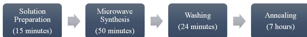
Figure 3.15. Time diagram for nano-particle production.
