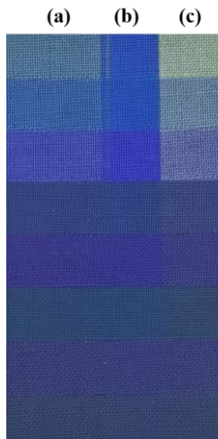
Figure 3.16. Blue Wool Scale for the samples tested. (a) 24 h, (b) no exposure and (c) 144 h.
