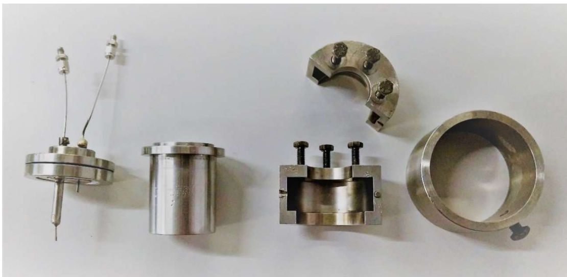
Figure 2.2. Picture of the reactor. From the right to the left: head of the reactor with a dip tube, cylinder, split ring closure rings with bolts, drop band.
