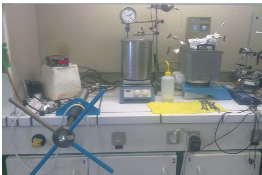
Figure 2.9. Picture of the screw injector assembled to the apparatus.
