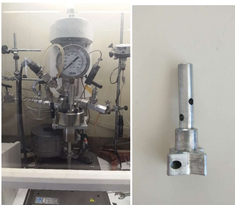
Figure 2.14. Photograph of the series 4591 micro Parr reactor installation on the left; picture of the stirring mixer.
