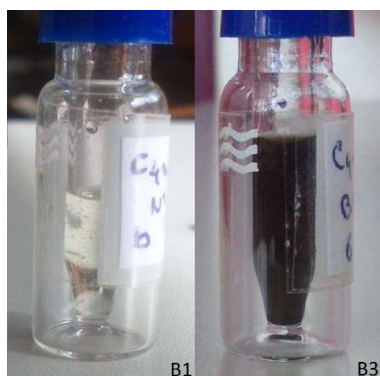
Figure 3.7. Picture of samples B1 (Ru(cod)methylallyl 2 in [C 4 mim][NTf 2 ], freshly prepared) and B4 (Ru(cod)methylallyl 2 in [C 4 mim][NTf 2 ], 2 days old).
