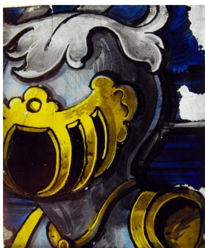
Figure 1.9 – In this 17 th century (?) stained-glass fragment (PNP2534) located at the Noble Hall of Pena National Palace, the detachment of the blue enamel paint from the base glass is visible. © Andreia Machado.
