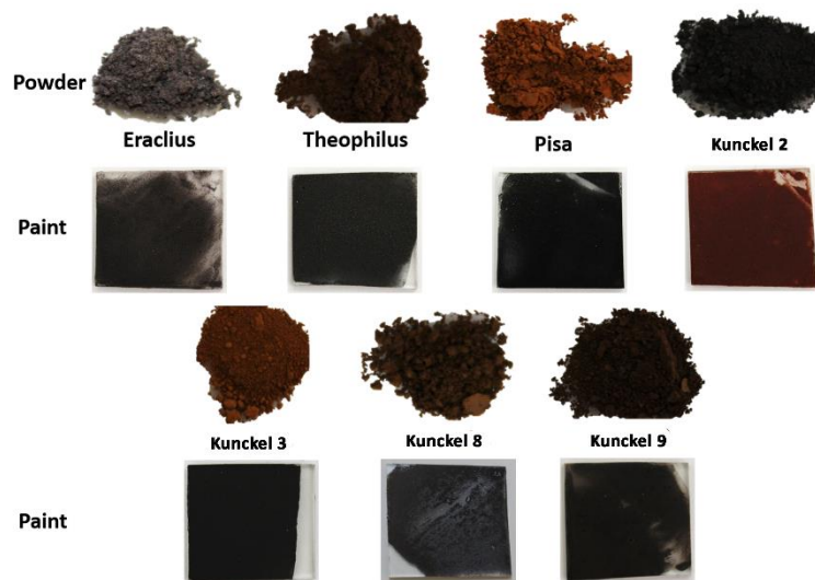
Figure 4.44 – The results obtained for the grisaille paint reproductions, both powder and paint samples.
