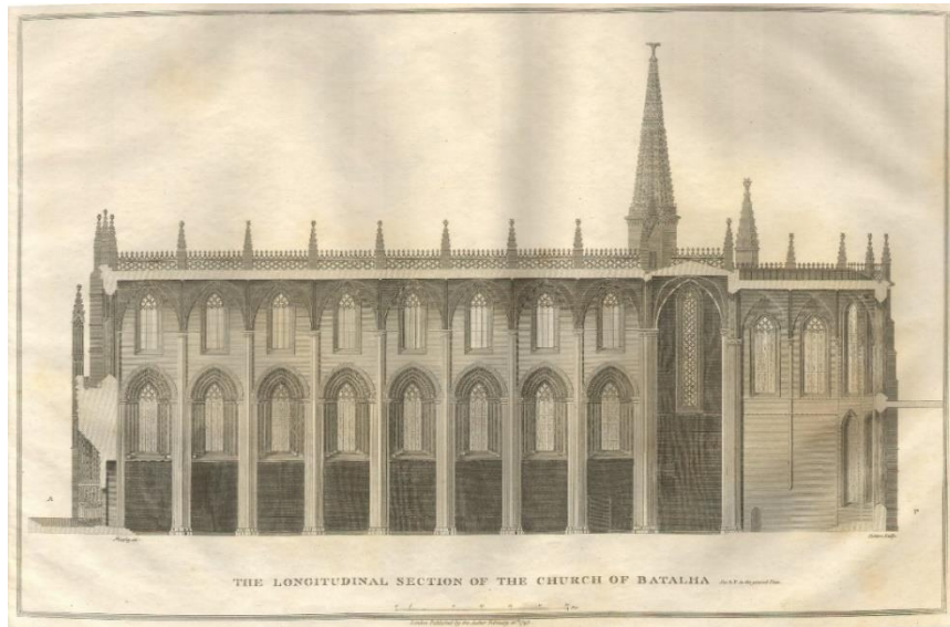
Figure 2.2 – Drawing from the longitudinal section of the church of Batalha Monastery by James Murphy.
