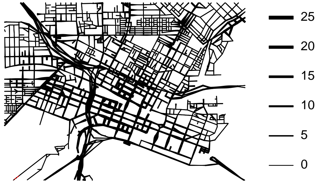
Figure 2.33: Intensity estimate in the Perth CBD using fixed-bandwidth uniform correction with automatically selected bandwidth \sigma = 0.091 km. Intensity values are proportional to line width.
