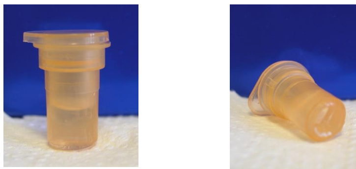
Figure 29 – Dialysis membrane after finishing the solubility assay of 0.45 mg of simvastatin.
