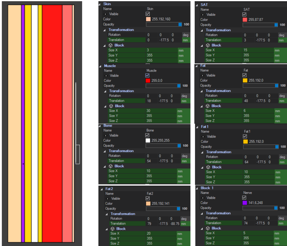
Figure 3.11: Multi-layered model. The area of each layer is 355 \times 355 \text{ mm}^2 .
