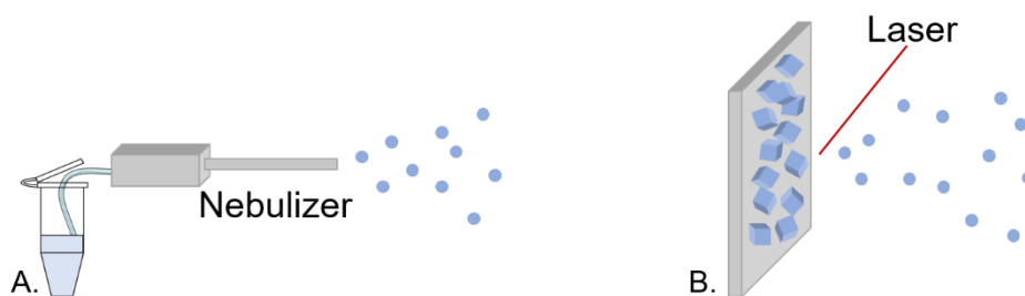
Figure 1.5: Depiction of two of the most common sources of ionization in mass spectrometry: A. Electrospray ionization (ESI) and B. Matrix-assisted laser desorption/ionization (MALDI). (Adapted from Aebersold et al. 57 )
