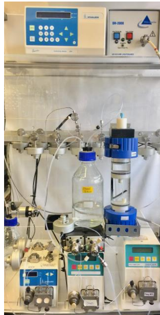
Figure 7 - One-Column analog SMB setup.
