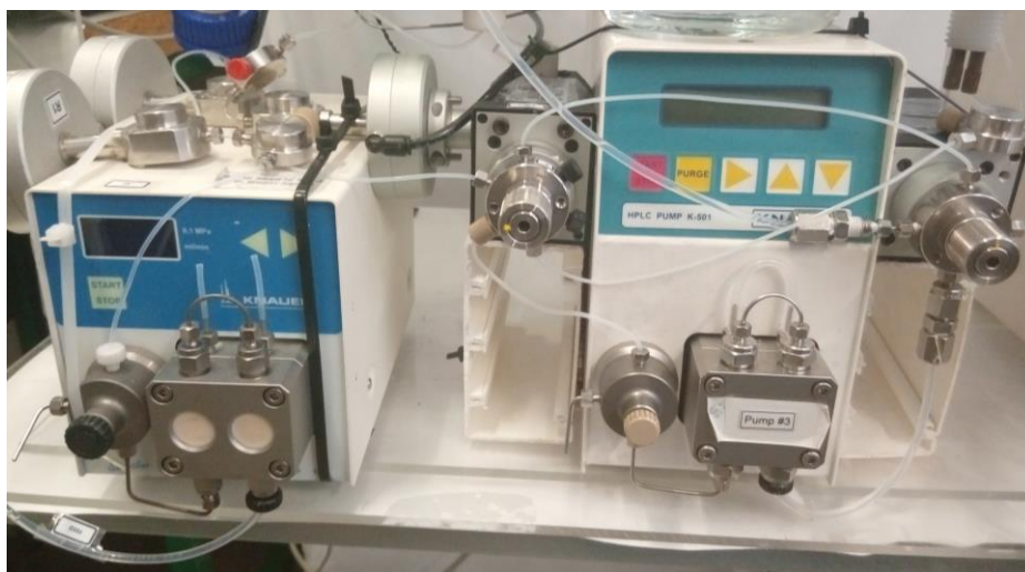
Annex 2 - Photo of the Knauer V5010 S100 Smartline pump (Pump F) and one of the Knauer WellChrom HPLC K501 pump (Pump E) along with the VICI Valco 2-position valves in the setup.
