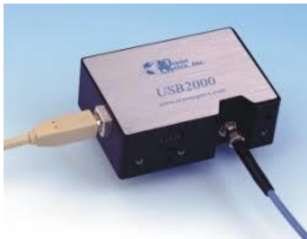
Annex 7 - Image of the OceanOptics USB2000 Spectrometer connected through a USB 2.0 Type B cable.
