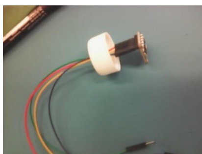
Figure 3.12- Temperature & humidity sensor adapted to the sample chamber's lid.
