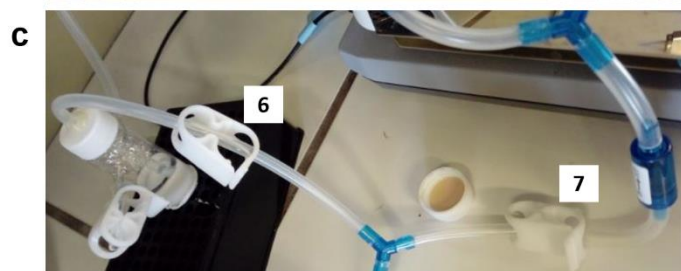
Figure 3.13- Experimental setup of the RH delivery system; (a) basic schematic, with exposure course is highlighted in bold; (b) and picture of the system; (c) manual system for alternating between exposure and recovery periods; (1) mass flow controller; (2) bubblers in series of supersaturated salt solutions; (3) first temperature & humidity sensor; (4) e-nose housing the array of hybrid gel thin films; (5) second temperature & humidity sensor; (6) clamp in exposure course; (7) clamp in recovery course.
