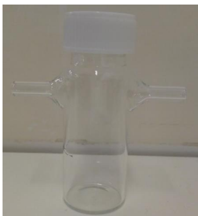
Figure 3.11- Tailor-made glass vial used as sample chamber and bubbler used in the e-nose experiments.
