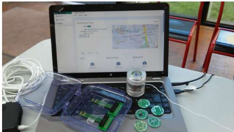
Figure 5.8: Data gathering, from the capsule into a computer, displayed in a graphical interface.
