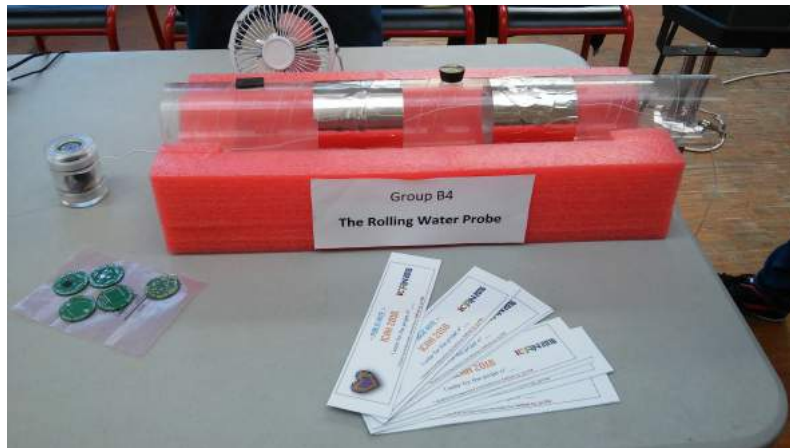
Figure B.10: Test setup, for demonstrate the prototype at work. The capsule will pass to an acrylic pipe to simulate the application environment.
