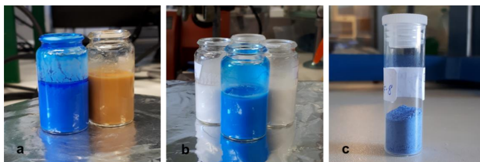
Figure 2.2. Preparation of IL@MOFs: (a) lidless ZIF-8 + IL + acetone vials being stirred, (b) heating up the mixture to ensure solvent evaporation, (c) sample after being dried.
