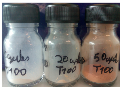
Figure 4.5: \text{TiO}_2 coated with 5, 20 and 50 MLD cycles using MC and 12BD.
