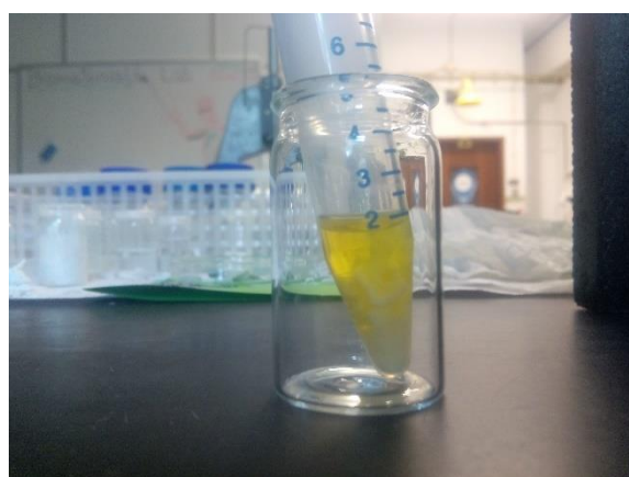
Figure 4.19 – Extract with pH indicator (Phenol red) after neutralization attempt. Yellow colour indicating an acid solution.
