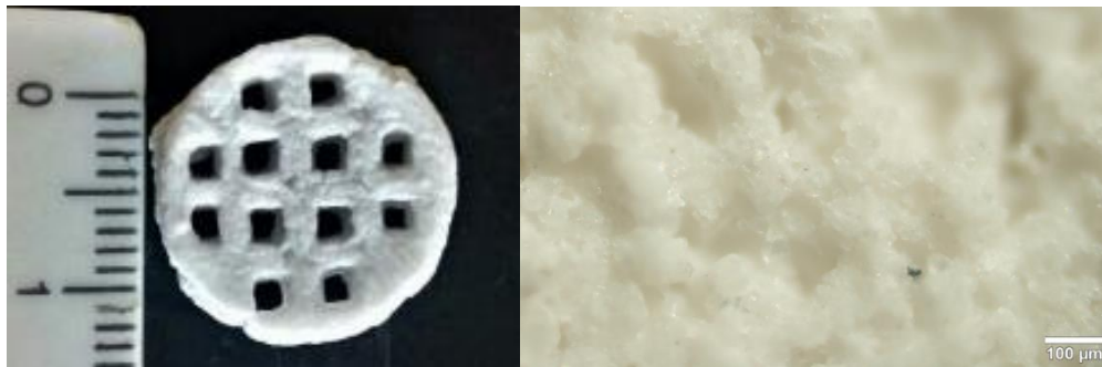
Figure 4.7 – Optical microscope image of the wall of a sintered 3D printed structure.
