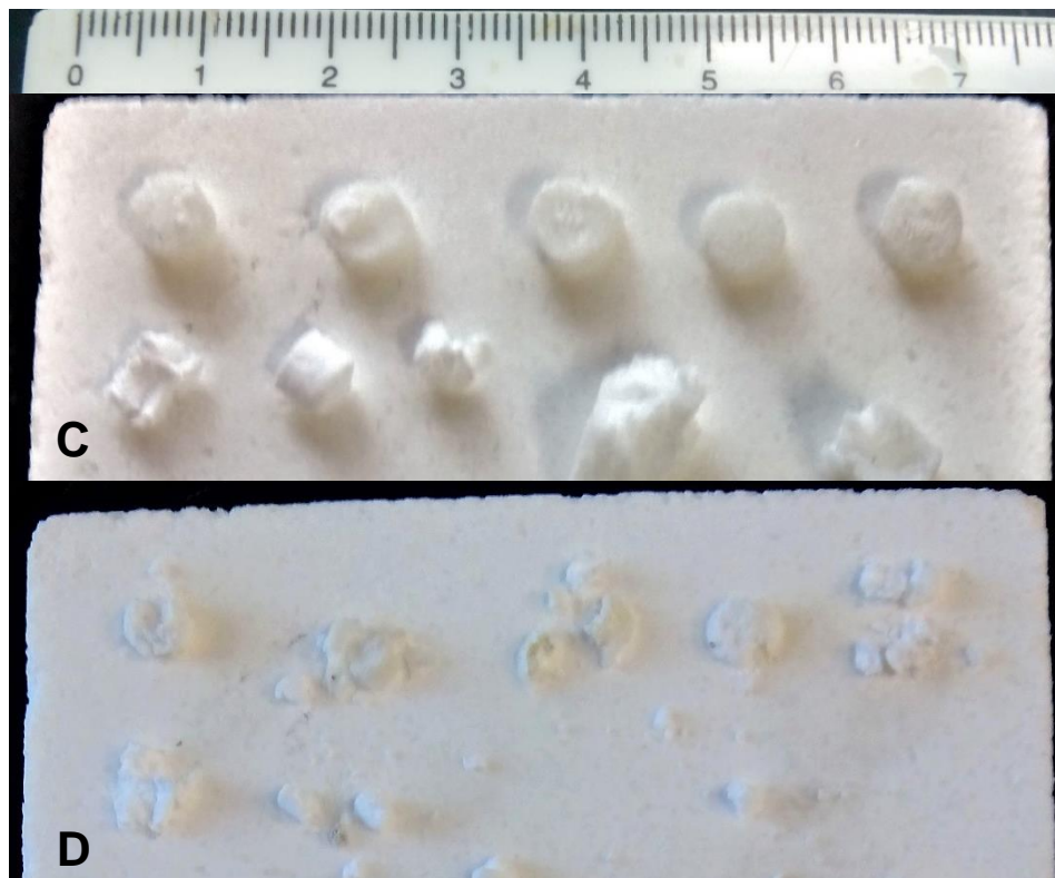
Figure 4.5 – Before (C) and after (D) sintering of the freeze dried samples.
